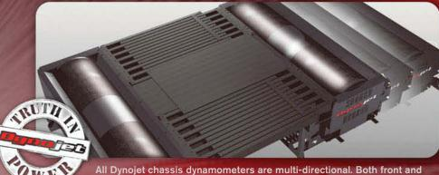
All Dynojet chassis dynamometers are multi-directional. Both front and rear wheel drive vehicles can be tested in either direction.
