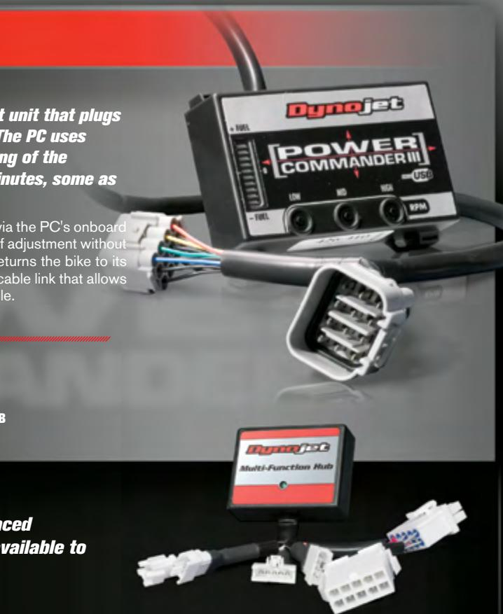
The Power Commander III USB is a fuel injection adjustment unit that plugs "inline" with the bike's stock ECU (electronic control unit). The PC uses original equipment style connectors, so no splicing or cutting of the harness is required. Most installations take less than 15 minutes, some as little as 5 minutes.
