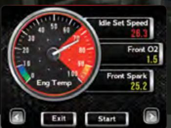
User defined visual alarms for any data channel (example, if knock exceeds 2 degrees, or if Cylinder Head Temp exceeds 280 degF, enable visual alarm).
